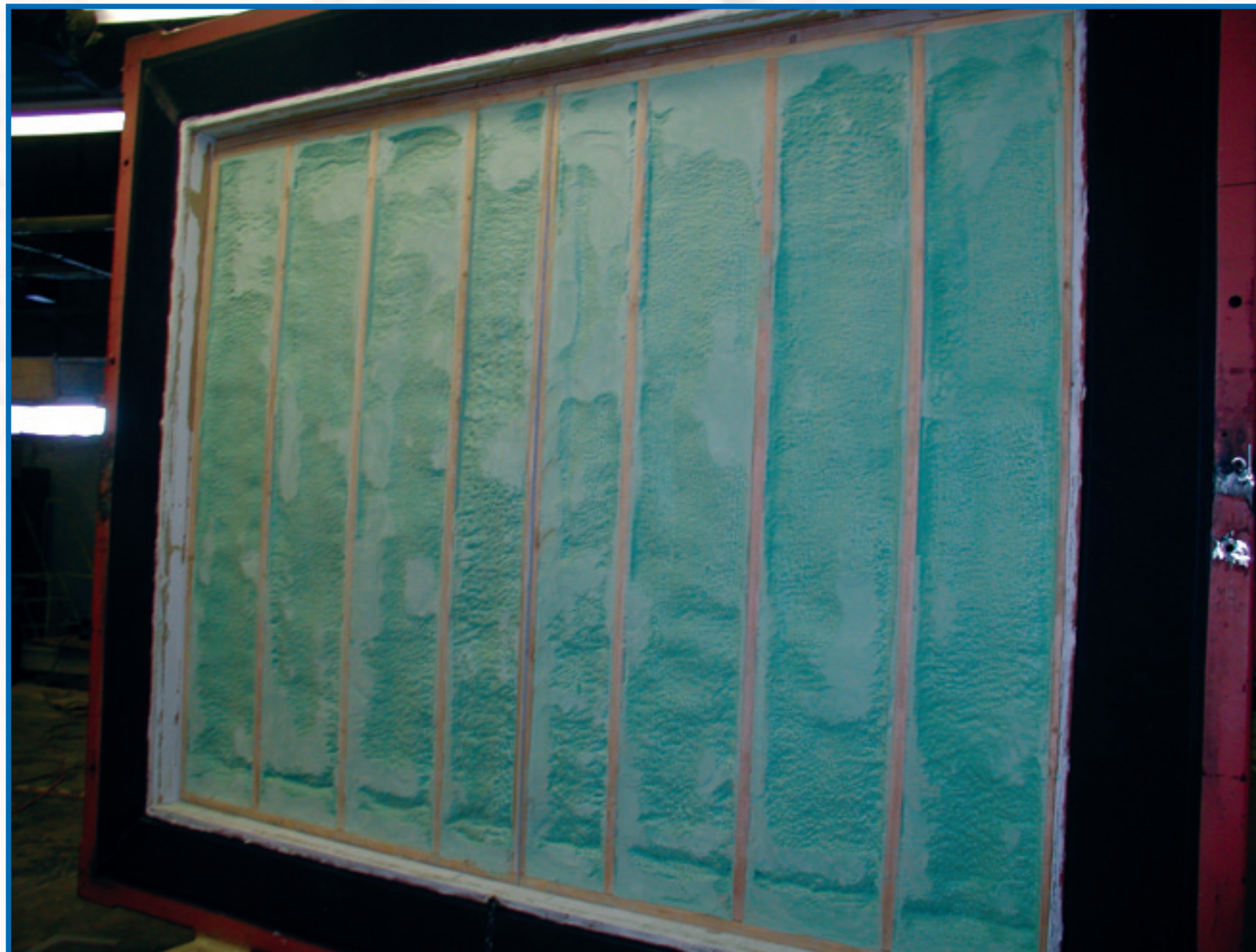
ASTM C1363: Interior side of SPF test wall
